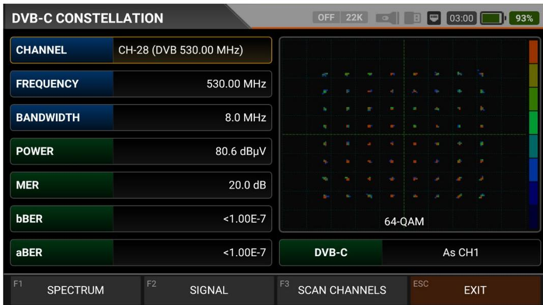
The constellation diagram shows in a graph the accuracy of the coordinates of the Digital I/Q symbols received at any given time. The colour scale, placed on the right side, provides a qualitative indication of the signal quality by grading the colours in proportion to the intensity of the dots concentrated in a particular area. The colour scale ranges from black (no symbol) to red (highest intensity).
