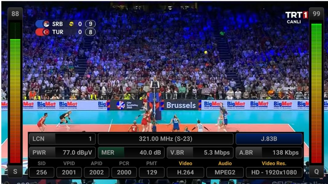
You can enlarge the image by touching it and pressing the LEVEL button to see both the image and the Signal levels, AV bitrate rates and PID values on the same screen.
