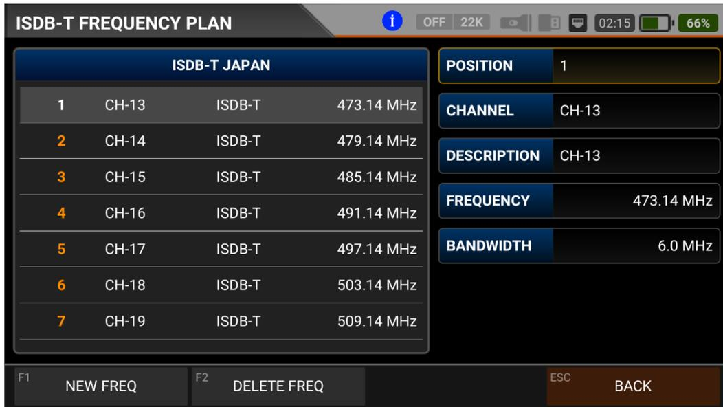
You can manually change these frequency plans on the device or via a PC program. You can access all parameters such as Frequency, BW, and TV system for each frequency.
