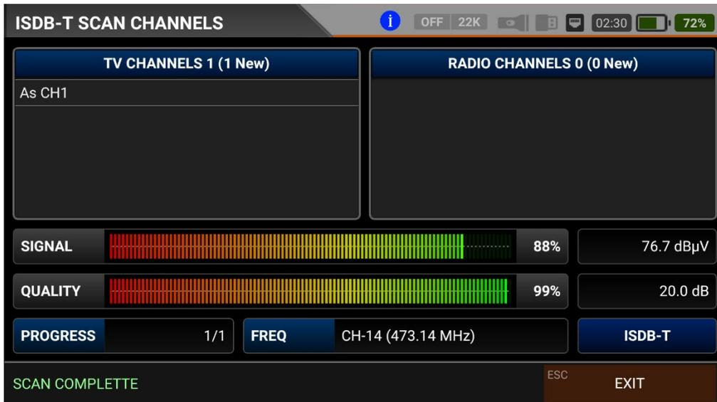
Scan Channels: You can search for TV channels suitable for your frequency plan in the ISDB-T band. You can then monitor and measure these channels.
