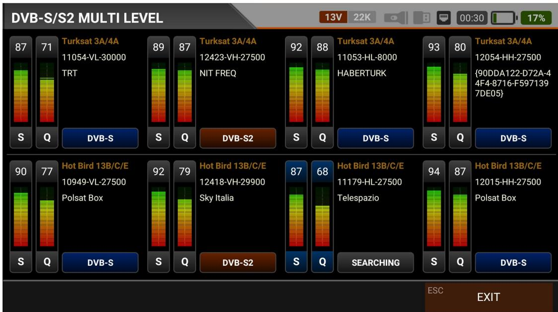
You can test the accuracy of Multiswitch and System assemblies by seeing all frequencies on the same screen. The device will sort the TPs on all satellites according to their VL/VH/HL/HL/HH polarity. This allows you to check the accuracy of 8 cables from 2 satellites in multiswitches.
