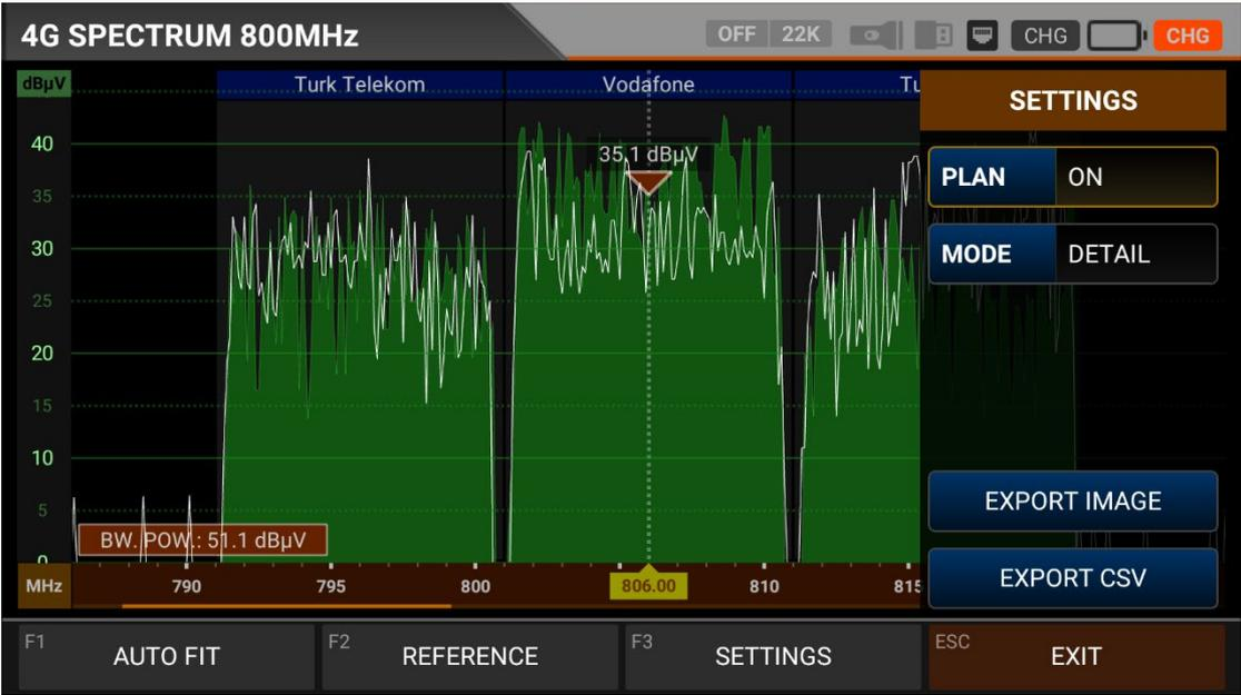
REFERENCE: You can SAVE the top points of the spectrum as a white line, and then you can RECALL them from memory in your subsequent measurements and re-install them with the same settings.
