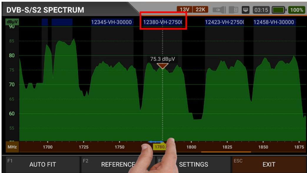
You can change the SPAN (frequency range) with the EDIT button on the spectrum screen or by using two fingers in the red area. If you enter the spectrum menu by selecting a frequency, you can see the selected TP frequencies and other TP frequencies of the same polarity in the red box. This allows you to control the entire TP frequency plan in the selected polarity.
