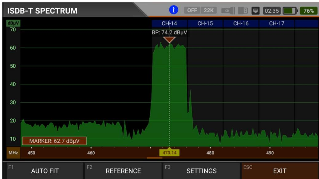
The device displays all ANALOGUE and DIGITAL carrier signals determined to be within the selected spectrum (frequency domain) when the DIGITAL SPECTRUM ANALYSIS measurement mode is switched. You can see the names of the channels in the green boxes at the top. You can see the Band Peak Power on the marker, and you can also see the instantaneous power of the marker line on the bottom left.
