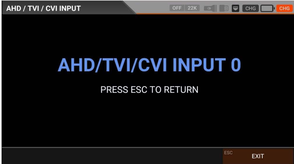
The device will count for 3 seconds and switch to CCTV mode when you select AHD/TVI/CVI. You can see the supported resolutions below.
