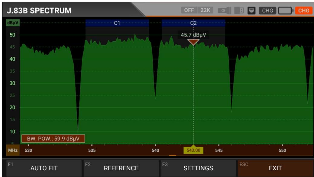
The device displays all ANALOGUE and DIGITAL carrier signals determined to be within the selected spectrum (frequency domain) when the DIGITAL SPECTRUM ANALYSIS measurement mode is switched. You can see the names of the channels in the green boxes at the top. You can see the Band Peak Power on the marker, and you can also see the instantaneous power of the marker line on the bottom left.
