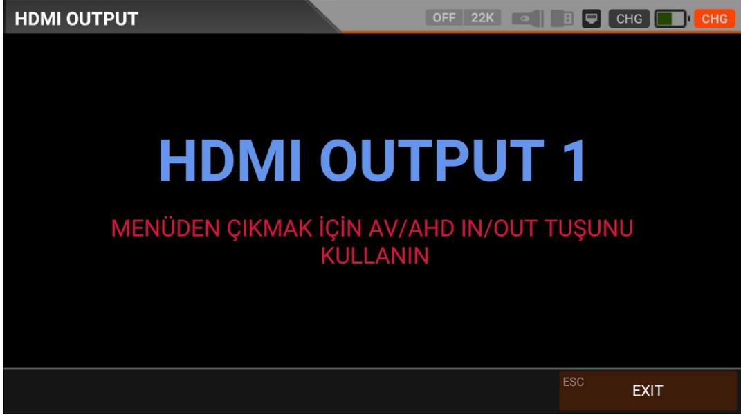
The device will count for 3 seconds, and you can test cables and TVs up to 4K resolution when you select HDMI OUT. Press AV/AHD/IN/OUT to exit from this mode to the MAIN MENU.
