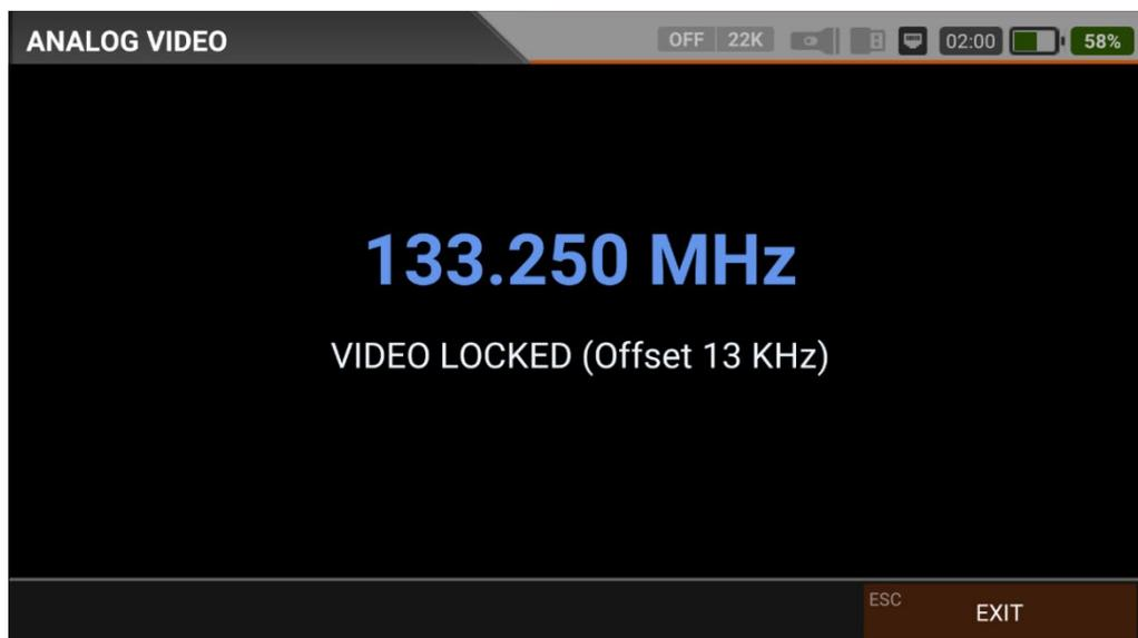
You can see the Analogue TV channels after locking to the frequency by touching the SHOW CHANNEL box at the bottom right. While watching Analogue TV channels, no menu function works; you can only exit Analogue TV with the ESC button.
