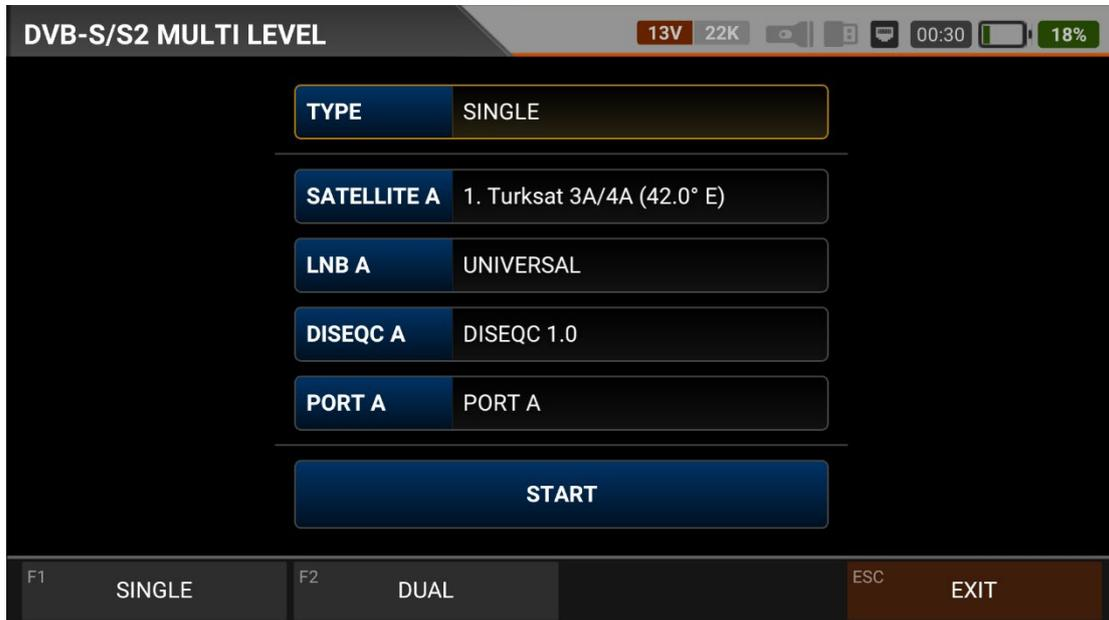
**SINGLE SATELLITE CONTROL:** Select SINGLE as the type and touch START after making the necessary SATELLITE settings. As shown in the screen below, the signal levels of 4 different frequencies from 1 satellite can be seen on the same screen. This allows you to check that the signal levels and antenna tuning are correct at all frequencies. You can look at the ports of the Quattro LNbs that supply the multiswitches one by one.
