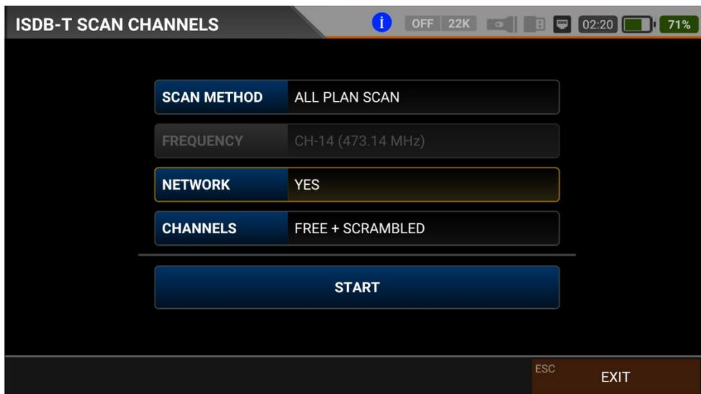
You can then start the scan channel process by touching the START box. In the scan channel screen, you can see which frequencies you scan and the signal values. It will show the newly found channels in white colour on the screen.
