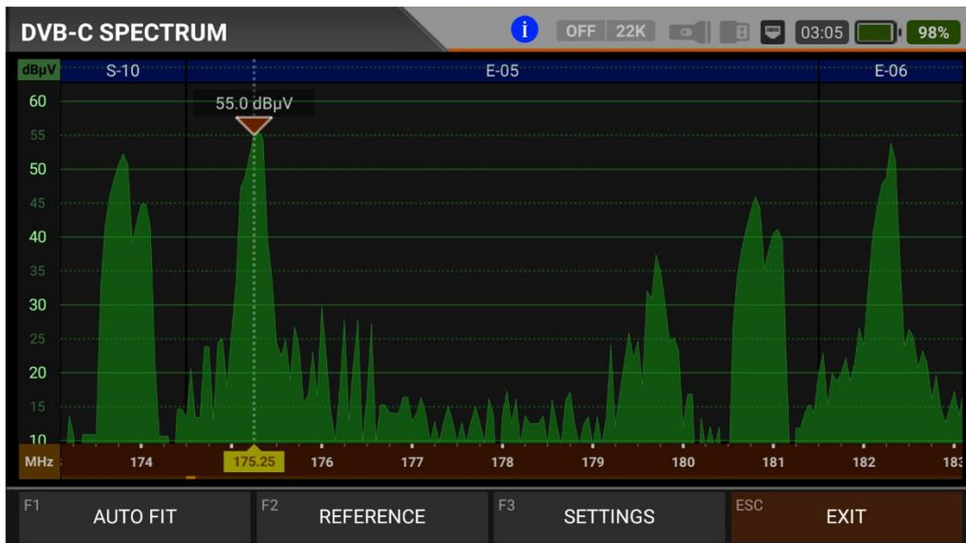
You can see the spectrum of a VHF terrestrial analogue cable TV channel on the screen above. You can access the Video-Audio-Colour spectrum detail of the channel you have measured by touching the Spectrum Box on the signal measurement screen.
