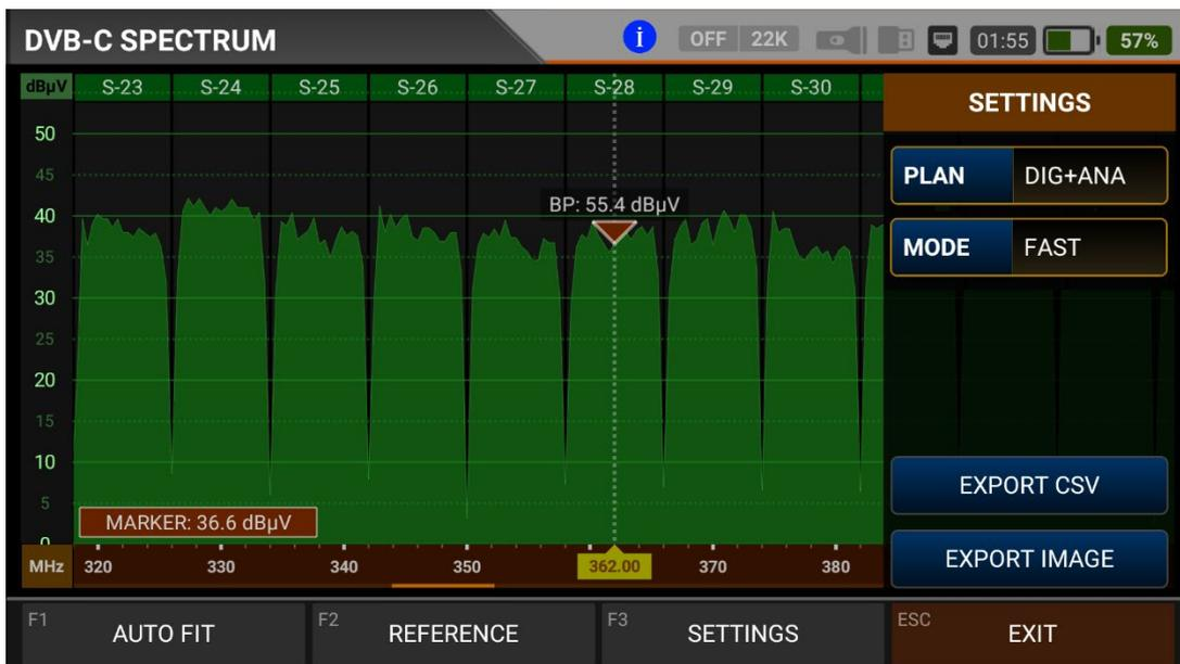
SETTINGS: This menu allows you to change the Tp Frequency Plan shown with blue bars to OFF/DIGITAL/ANALOGUE/DIG+ANA. This allows you to restrict the transmitting system you want to appear on the screen. You can change the operating mode of the spectrum quickly and precisely.
