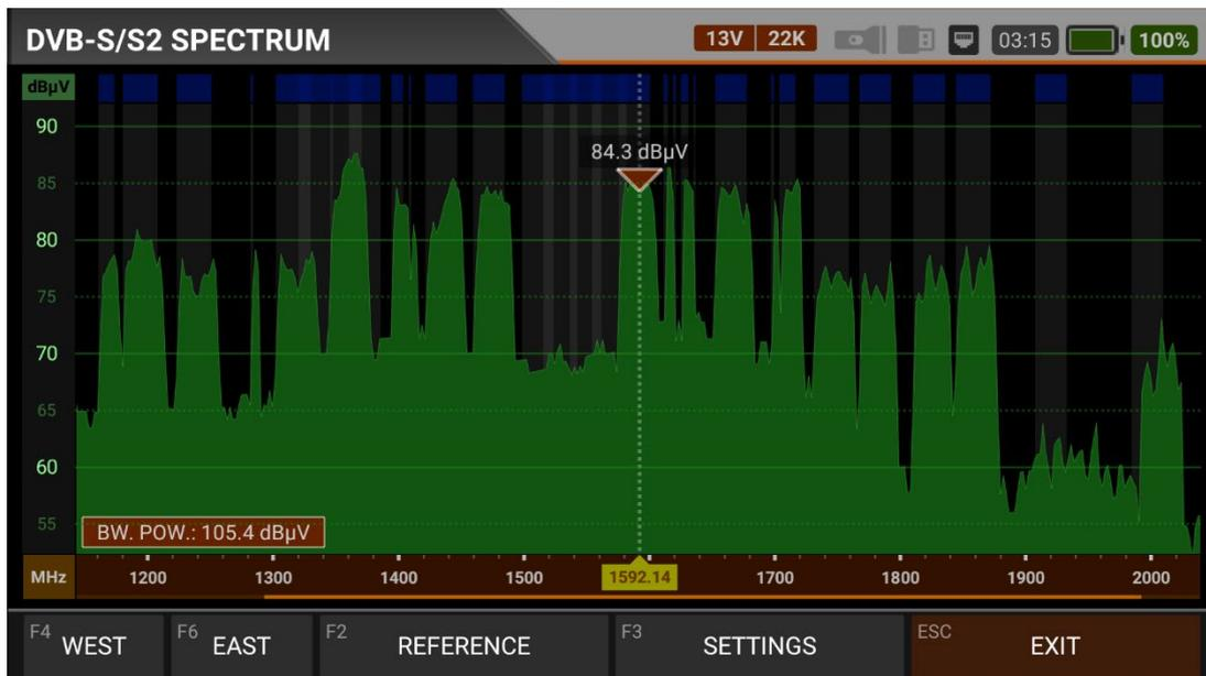
Firstly, select Diseqc 1.2 Motor from the DISEQC TYPE section of the Spectrum Analysis menu where you want to use the Diseqc-C engine feature. You can see the SPECTRUM levels, and at the same time, you can manually rotate your Diseqc 1.2 Motor to EAST / WEST by pressing the EAST / WEST boxes.
