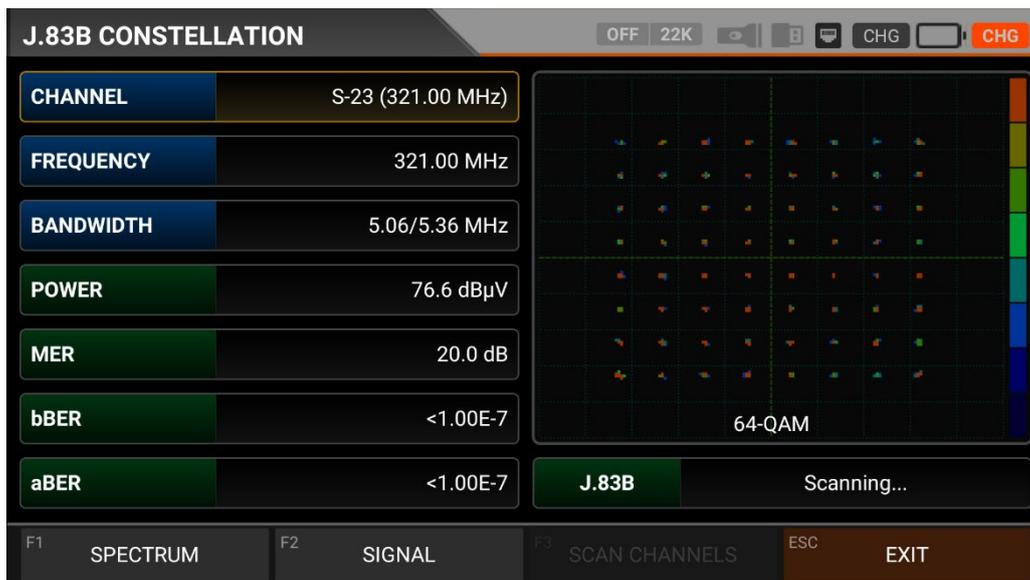
The constellation diagram shows in a graph the accuracy of the coordinates of the Digital I/Q symbols received at any given time. The colour scale, placed on the right side, provides a qualitative indication of the signal quality by grading the colours in proportion to the intensity of the dots concentrated in a particular area. The colour scale ranges from black (no symbol) to red (highest intensity).
