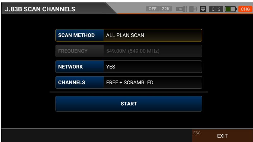
You can then start the scan channel process by touching the START box. In the scan channel screen, you can see which frequencies you scan and the signal values. It will show the newly found channels in white colour on the screen.
