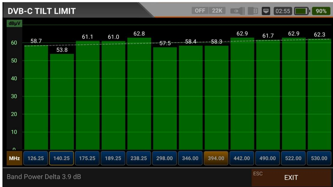
Tilt/Limit list testing is an effective solution to check the regularity of the cable system and further attenuation of the wave at high frequencies. AS07STCA can get the levels of 12 channels and easily observe the measurement result and graph. You can select the first six frequency starts of the group and the last six frequencies from the end of the group. You can then check the slope of the group and arrange the amplifiers and elements in the cable line according to this slope.
