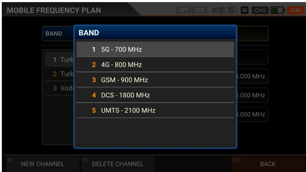
Your device keeps a Frequency Plan for each GSM system in its memory to be used in repeater installations. You can assign Names for your frequency plans.
