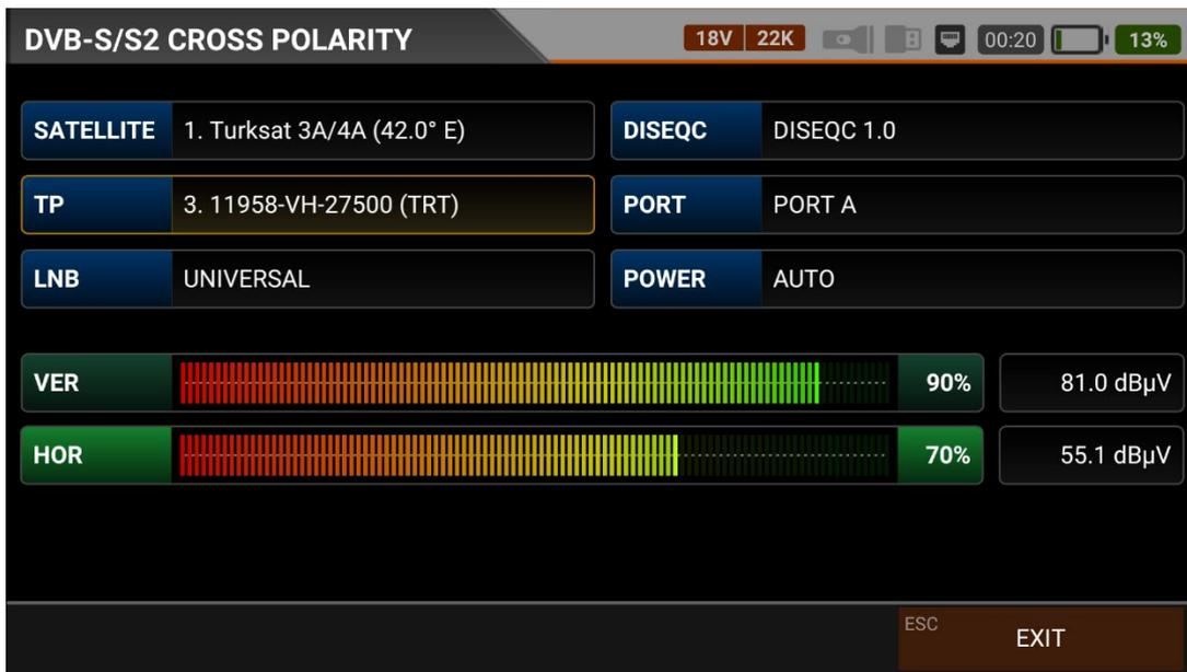
The purpose of this menu is to adjust the LNB according to the signal level at the opposite polarity of the selected frequency. We set it so that the top signal level is the highest. If the signal at the bottom moves in the same direction as the signal at the top, both should be set to the highest or if it moves in the opposite direction, the upper signal should be set to the highest and the lower signal to the lowest.
