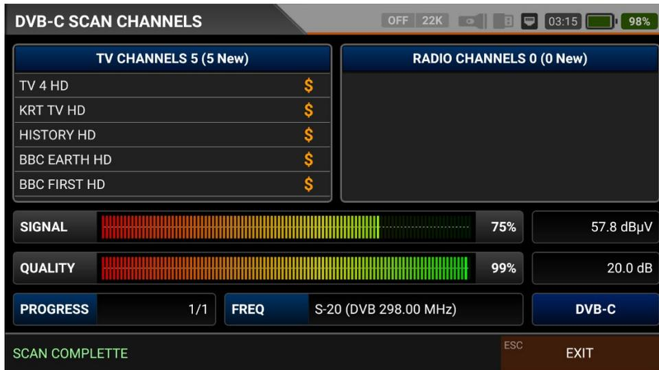
Scan Channels: You can search for TV Channels suitable for your frequency plan in the DVB-C band. You can then monitor and measure these channels.
