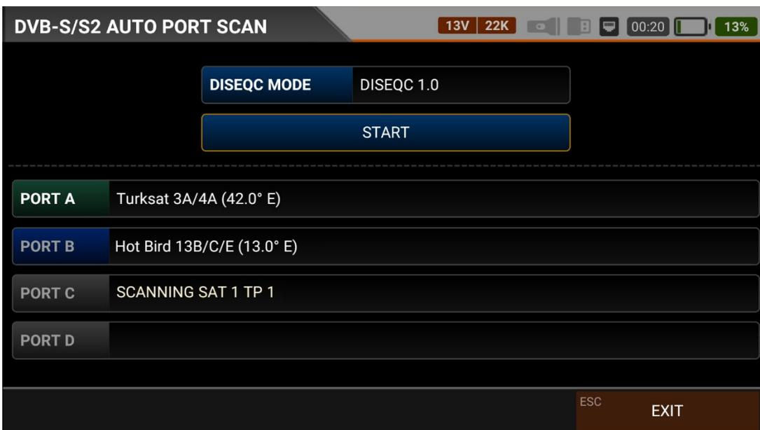
We can see which satellite the Dish Antenna is facing or which satellites are connected to which ports of our Diseq-C Switch. This way, you don't have to go near the antenna or find cables. Diseq-C 1.0 and Diseq-C 1.1 protocols are installed and ready to use inside your device. You can use it in all 4 and 8 Diseq-C switches.
