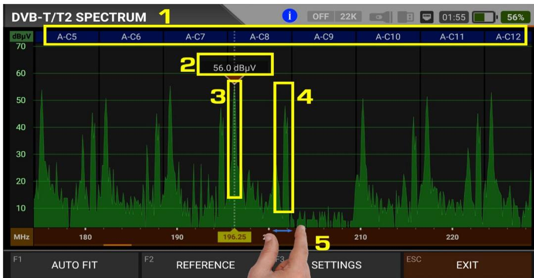
The device displays all ANALOGUE and DIGITAL carrier signals determined to be within the selected spectrum (frequency domain) when performing ANALOGUE SPECTRUM ANALYSIS measurement. You can see the following information on the screen according to the frequency plan we have previously selected.
