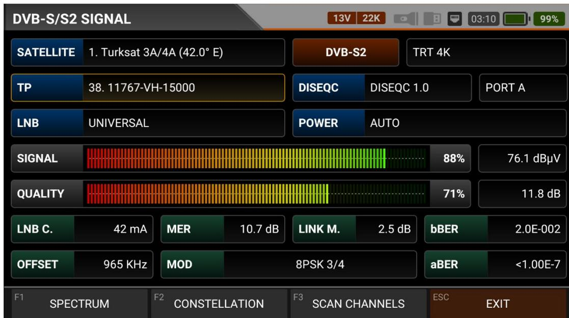
Your AS07STCA-4K is capable of measuring DVB-S/S2 - QPSK/8PSK signals. It can also show SD-HD-FHD-4K TV channels. You can select the satellite, transponder, Diseqc Type and lnb type you want to adjust your dish antenna or check the signal levels and see the signal values on the screen. You can also make more detailed settings with the SPECTRUM and CONSTELLATION box.
