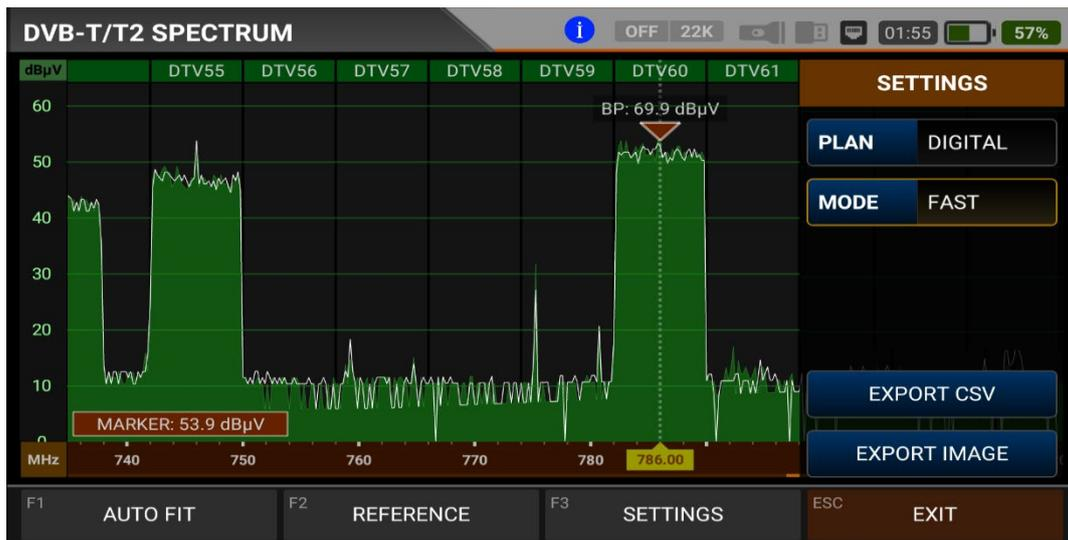
SETTINGS: This menu allows you to change the Tp Frequency Plan shown with blue bars to OFF/DIGITAL/ANALOGUE/DIG+ANA. This allows you to restrict the transmitting system you want to appear on the screen. You can change the operating mode of the spectrum quickly and precisely.
