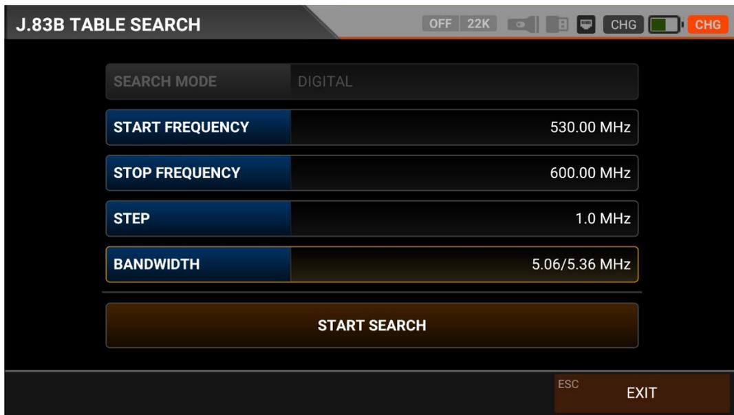
The AS07STC utilizes the channel scan function to quickly test the regularity and gain of the Cable TV system. You can select the start and end frequencies with the step range, and you can scan signals in the whole band with one of the 5.06/5.36 or 5.60Mhz bandwidths. You can check the signal values of all TPs using the TABLE MEASUREMENT menu when you have completed the system setup or when you go to service the subscriber.
