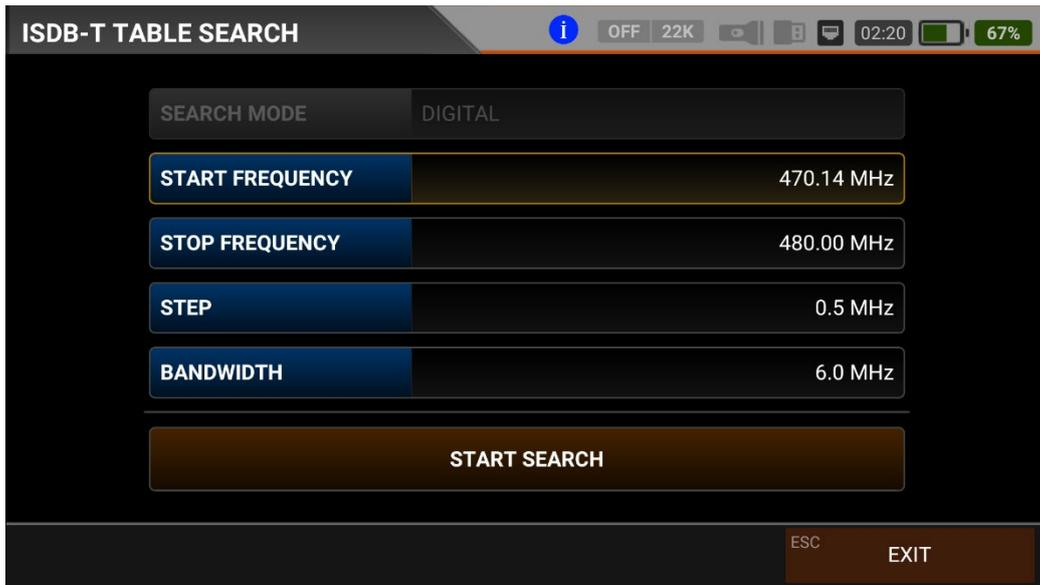
The AS07STC utilizes the channel scan function to quickly test the regularity and gain of the Cable TV system. You can select the start and end frequencies with the step range, and you can scan signals in the whole band with one of the 6/7/8Mhz bandwidths. You can check the signal values of all TPs using the TABLE MEASUREMENT menu when you have completed the system setup or when you go to service the subscriber.
