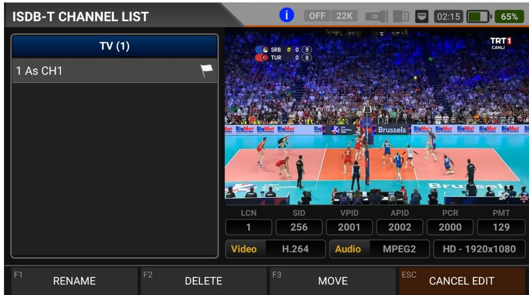
You can touch on the EDIT box and then perform the CHANGE NAME / DELETE CHANNEL and MOVE CHANNEL process. You can enter the number of the new position to move the channels to when you touch on a Channel or touch all the channels you want to move in BULK and press the MOVE box. Single channel and batch channels will be transferred to the new position, respectively.
