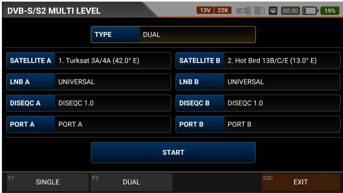
**DUAL SATELLITE CONTROL:** Select DUAL as the type and touch the START box after making the necessary SATELLITE settings. As shown in the screen below, the signal levels of 8 different frequencies from 2 satellites can be seen on the same screen.
