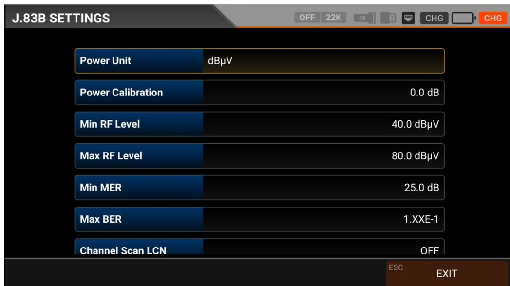
**Power Unit:** You can see the signal levels on the display in dBuV/dBm/dBmV units.
