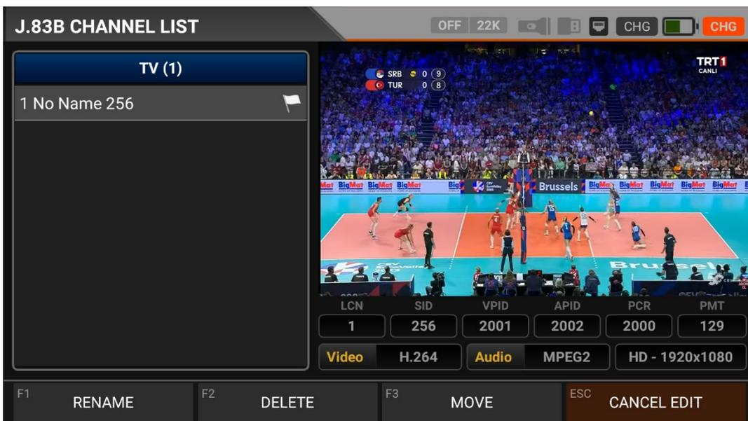
You can touch on the EDIT box and then perform the CHANGE NAME / DELETE CHANNEL and MOVE CHANNEL process. You can enter the number of the new position to move the channels to when you touch on a Channel or touch all the channels you want to move in BULK and press the MOVE box. Single channel and batch channels will be transferred to the new position, respectively.
