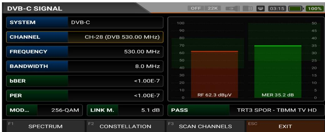
**SYSTEM:** It can be selected as ANALOGUE TV / DVB-C separately or ATV+DTV together in the frequency plan. This will display the frequencies of this system on the screen. It will make your installations faster.
