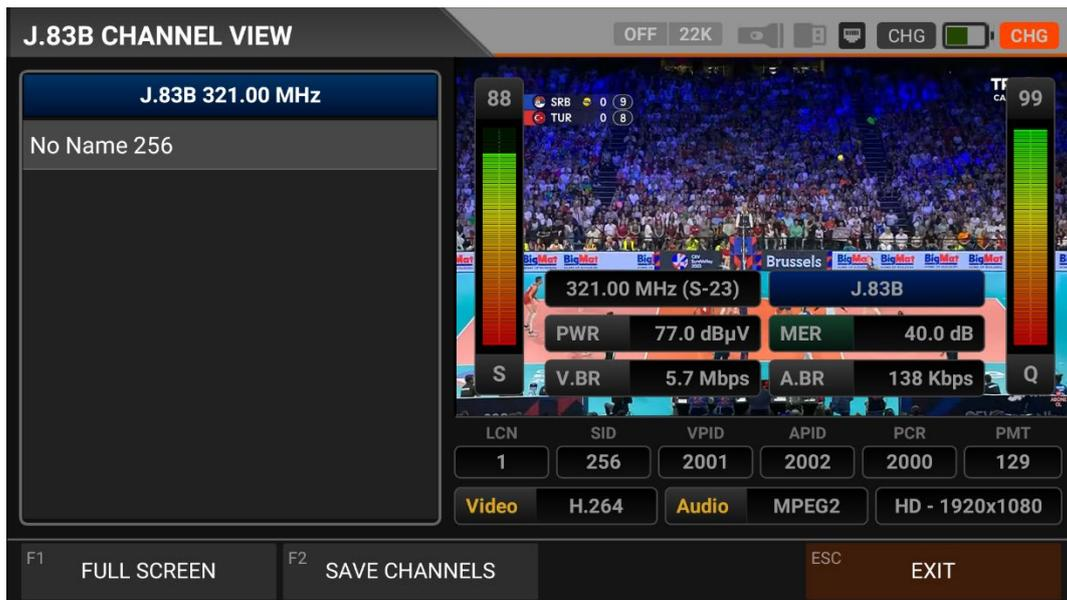
You can bring it to the screen by touching the CHANNEL LIST from the J.83B MENU. You can select, delete, and relocate individual TV and Radio channels in the Channel List menu. You can select channels from the left side. You can see the list of radio channels on the screen with the TV / RADIO button.
