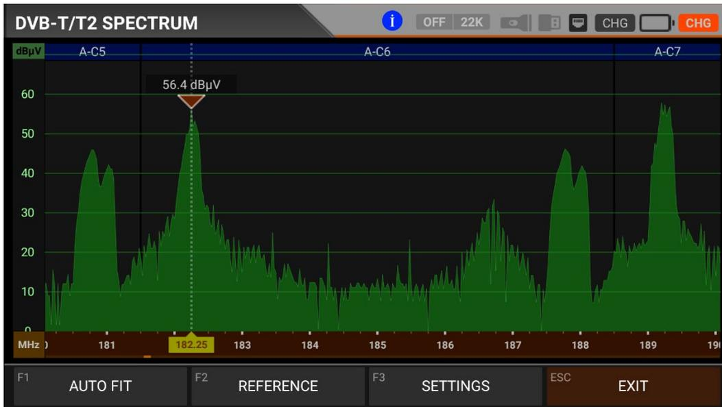
You can see the spectrum of a terrestrial analogue TV channel on the screen above. You can access the Video-Audio-Colour spectrum detail of the channel you have measured by touching the Spectrum Box on the signal measurement screen.
