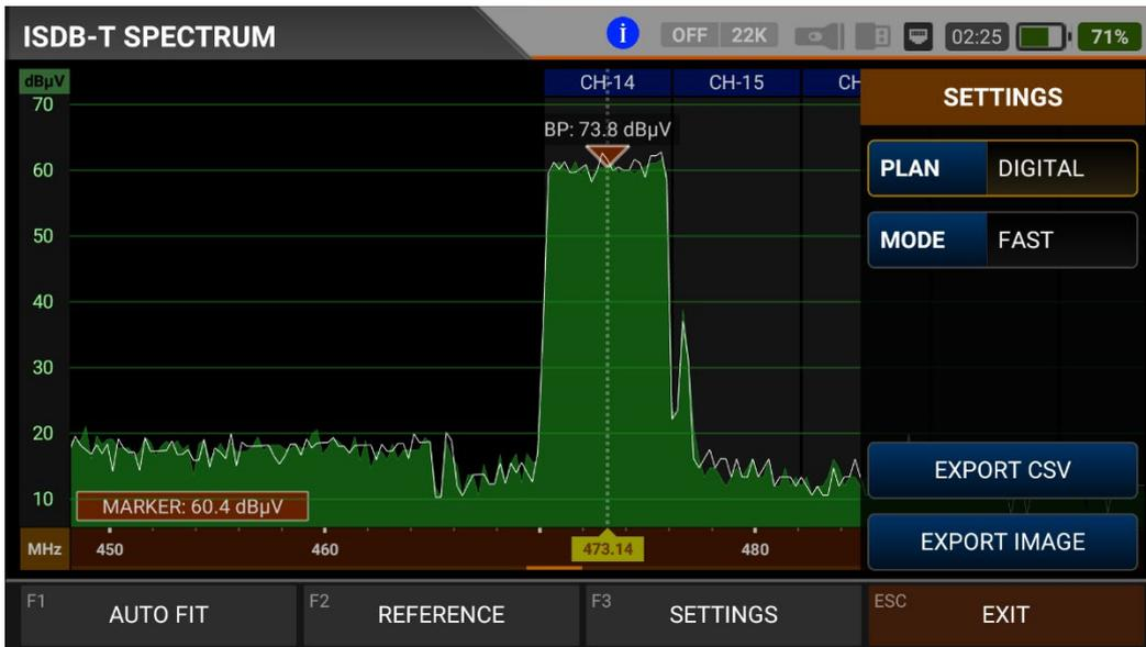
SETTINGS: This menu allows you to change the Tp Frequency Plan, indicated by the blue bars, OFF/ON. This allows you to restrict the transmitting system you want to appear on the screen. You can change the operating mode of the spectrum quickly and precisely.
