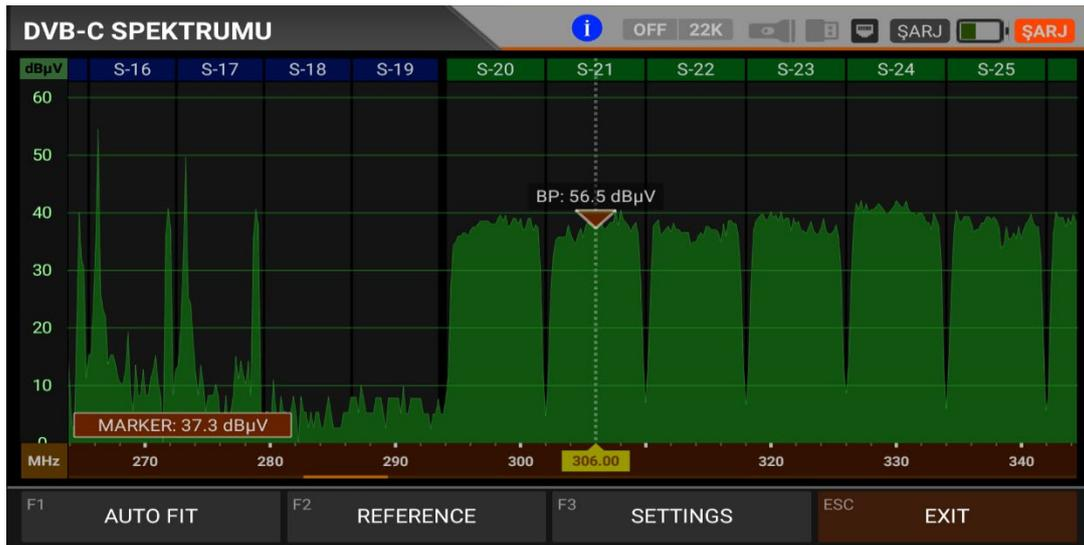
The device displays all ANALOGUE and DIGITAL carrier signals determined to be within the selected spectrum (frequency domain) when the DIGITAL SPECTRUM ANALYSIS measurement mode is switched. You can see the names of the channels in the green boxes at the top. You can see the Band Peak Power on the marker, and you can also see the instantaneous power of the marker line on the bottom left.
