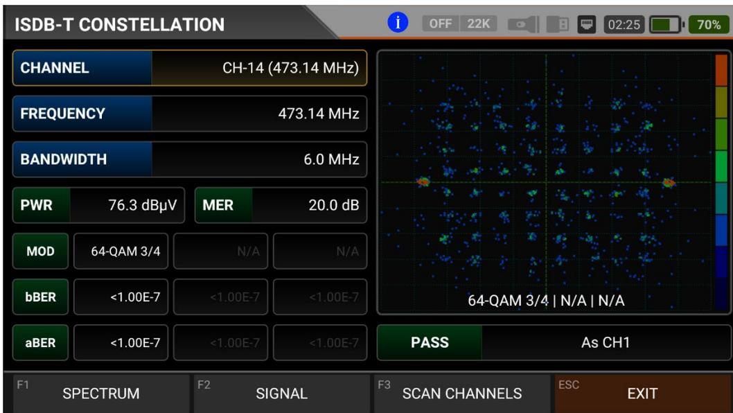
The constellation diagram shows in a graph the accuracy of the coordinates of the Digital I/Q symbols received at any given time. The colour scale, placed on the right side, provides a qualitative indication of the signal quality by grading the colours in proportion to the intensity of the dots concentrated in a particular area. The colour scale ranges from black (no symbol) to red (highest intensity). It shows three different modes at the same time.
