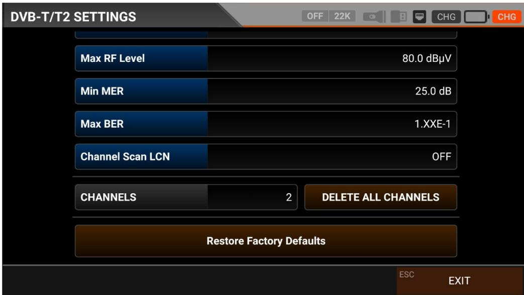
Min MER: When the MER value drops below this level, the device will not confirm that the installation was done correctly.
