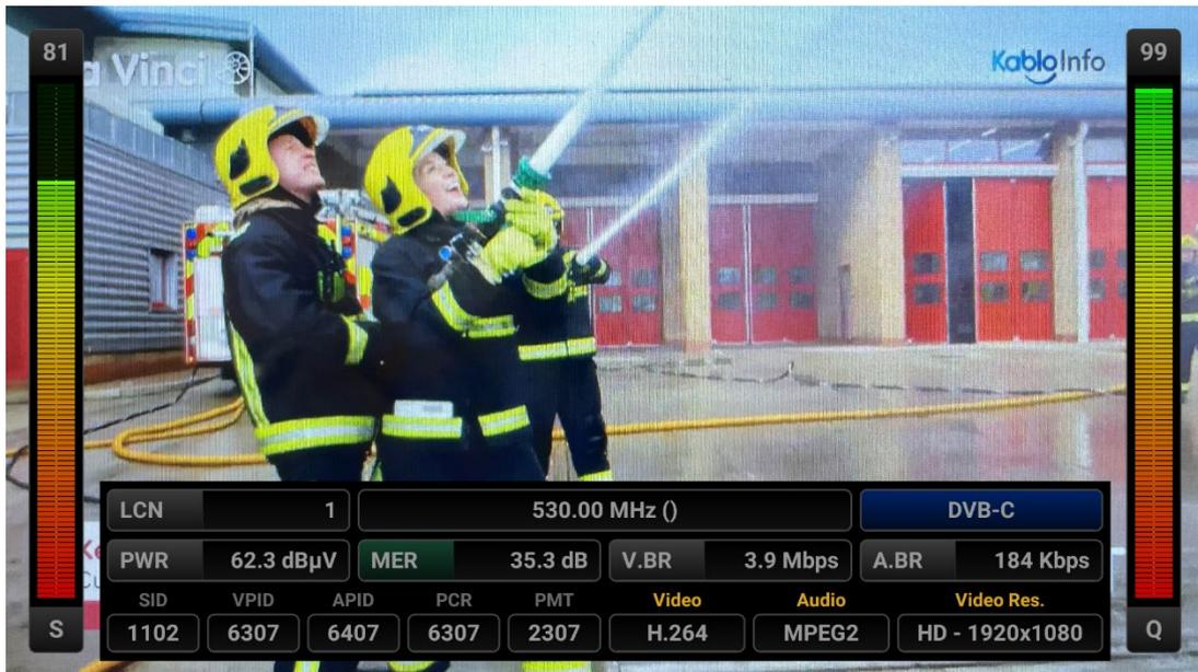
You can enlarge the image by touching it and pressing the LEVEL button to see both image and signal levels, AV bitrate rates and PID values on the same screen.
