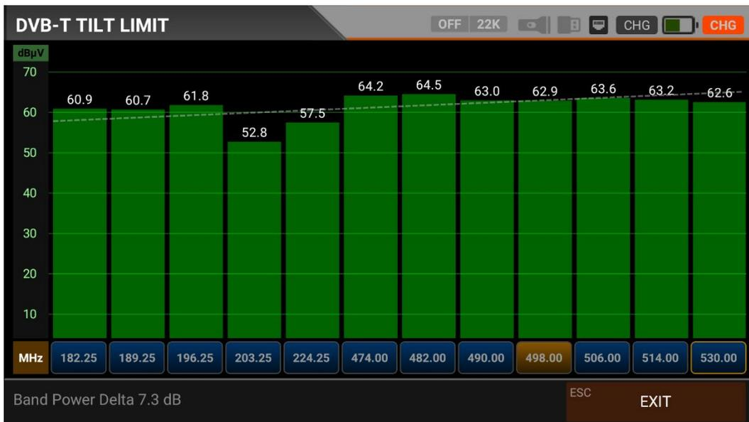
Tilt/Limit list testing is an effective solution to check the regularity of the cable system and further attenuation of the wave at high frequencies. AS07STCA can get the levels of 12 channels and easily observe the measurement result and graph. You can select the first six frequency starts of the group and the last six frequencies from the end of the group. You can then check the slope of the group and arrange the amplifiers and elements in the cable line according to this slope.
