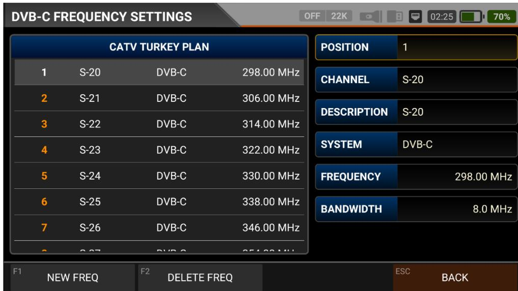
You can manually change these frequency plans on the device or via a PC program. You can access all parameters such as Frequency, BW, TV, and system for each frequency.
