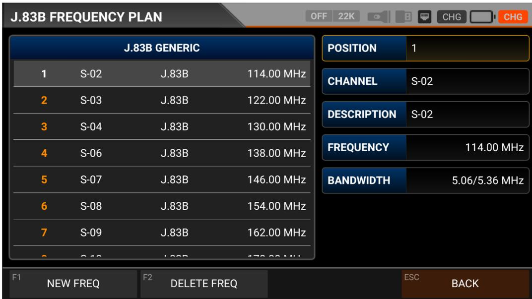
You can manually change these frequency plans on the device or via a PC program. You can access all parameters such as Frequency, BW, and TV system for each frequency.
