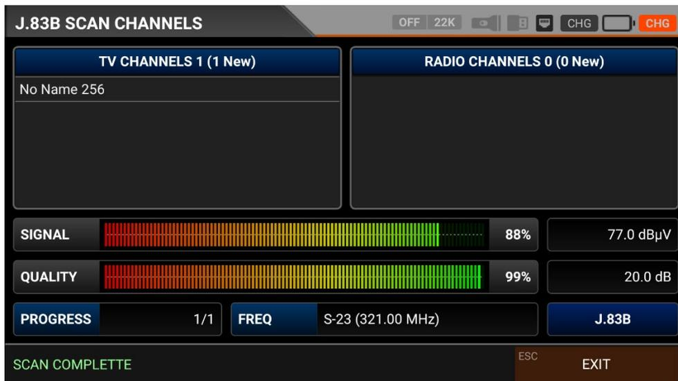
Scan Channels: You can search for TV Channels suitable for your frequency plan in the J.83B band. You can then monitor and measure these channels.
