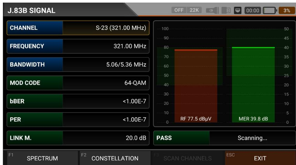
You can select the frequency at which you want to measure the J.83B (Annex B) signal or look at the signal levels and see the signal values on the screen. You can quickly switch to other measurement menus related to the frequency you have measured from the SPECTRUM, CONSTELLATION and CHANNEL SEARCH boxes at the bottom. Detailed information on Spectrum Analysis and Constellation properties will be given on the following pages.
