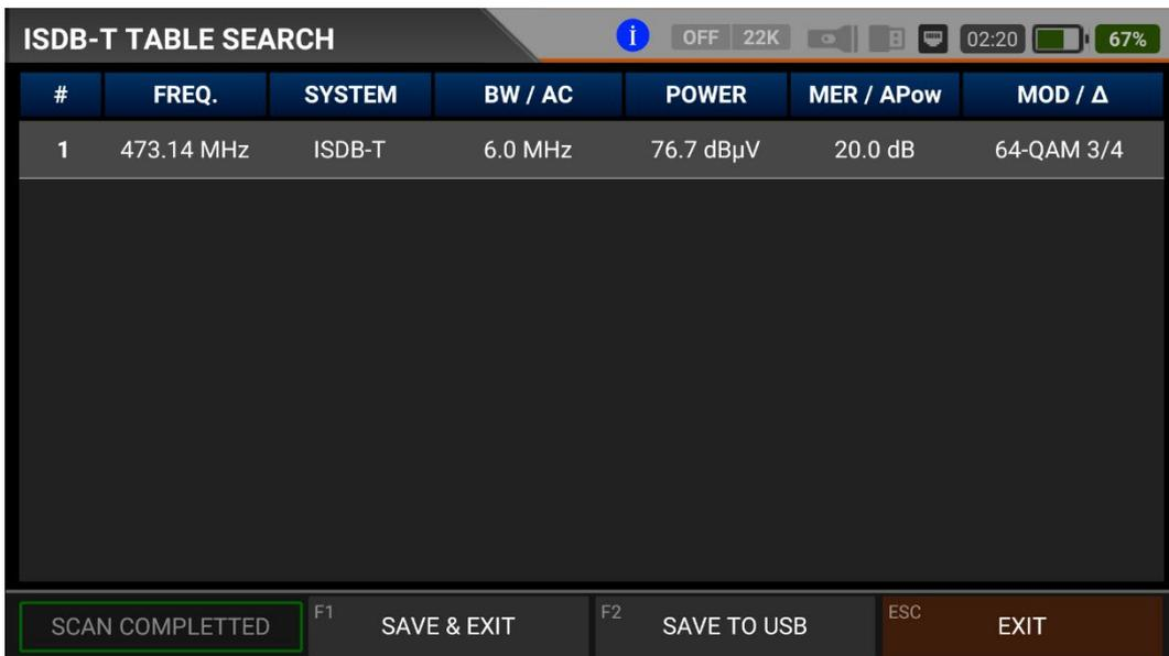
You can see which channel in the entire plan has a problem and compare frequencies. You will see the tables in the pictures after scanning all frequencies. You can save the entire table to USB with the "SAVE TO USB" button and save the measurement to the frequency plan used after all operations are finished.
