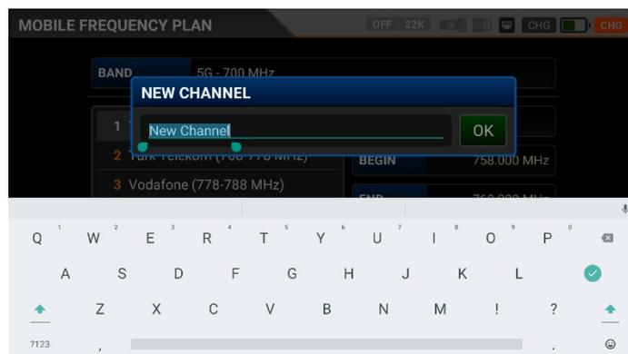
You can manually change the 5G-4G-3G-GSM1800-GSM900 frequency plans on the device or via a PC program. Frequency range and bandwidth must be entered for each operator band.
