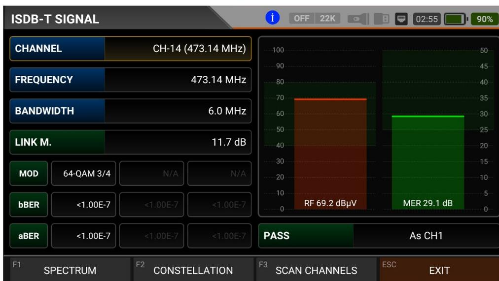
You can select the frequency at which you want to measure the ISDB-T signal or look at the signal levels and see the signal values on the screen. You can quickly switch to other measurement menus related to the frequency you have measured (473.143MHz frequency should be entered as 473.14MHz in the device) from the SPECTRUM,
