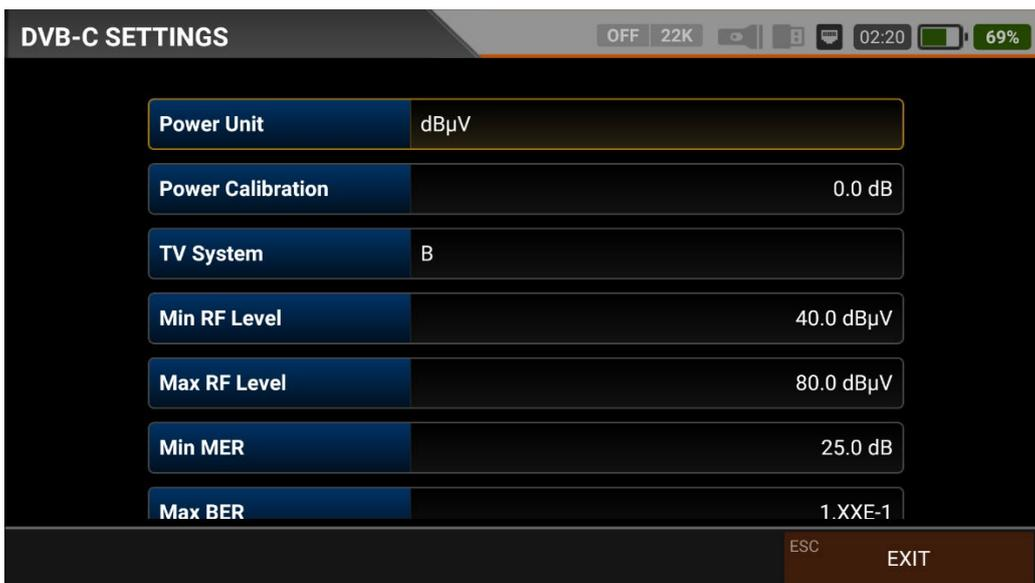
**Power Unit:** You can see the signal levels on the display in dBuV/dBm/dBmV units.
