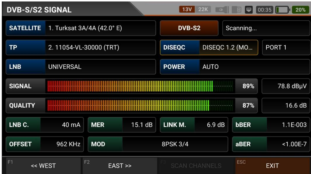
MER (Modulation Error Rate) is a metric used to measure the performance of the digital modulation of the signal in the communication system. MER is measured between 0-20db to check the ideal level of the signal after effects such as noise, low aspect ratio, phase noise, carrier suppression, distortion, etc., in our DVB-S/S2 device.
