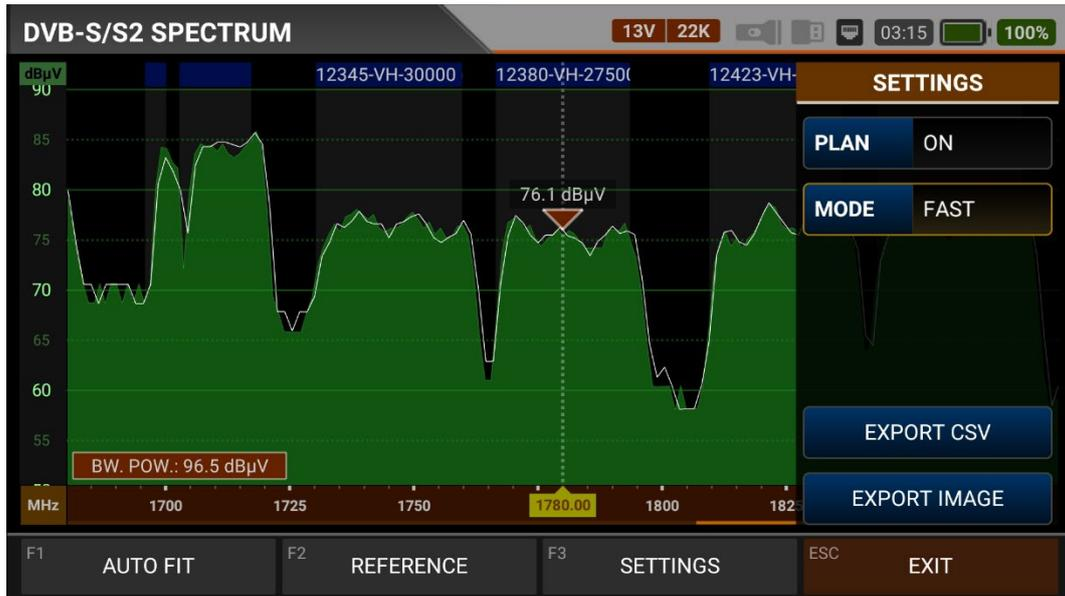
SETTINGS: This menu allows you to turn on/off the Tp Frequency Plan indicated by the blue bars. You can change the operating mode of the spectrum quickly and precisely. You can export the spectrum display as a \*.CSV file and as an IMAGE file to USB.
