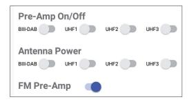
Recommendation: Turn on the pre-amplifier only when the input signal level is too low (below 60 dBµV). Users may consult the automatic power level measurement of the input signal when adding a channel on the ONE Compact.
