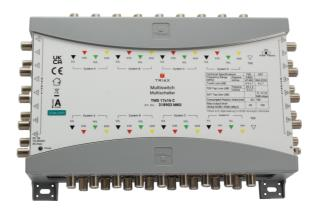
Cascade multiswitch for 4 Satellite positions with 17 inputs and 17 trunk outputs, suitable for distributing satellite and terrestrial signals in small to large sized systems. Available with 16 subscriber outputs and powered by the TMS PSU external power supply either directly or via the SAT trunk lines.
