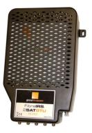
The two FibreIRS 2SATGTU's have been designed to output 8 satellite polarities, DTT, FM and DAB from a single optical input. Two versions available, Quad with 4 universal IF outputs with terrestrial available on each with DiSEqC commands used to switch between the two satellites. Quatro version has 8 fixed polarity IF outputs and a separate terrestrial connector
