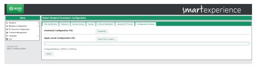
After that, push Upload button. A message will appear, indicating configuration is being applied. After some seconds, the configuration will have been applied and the browser will redirect you to the Site identification screen.
