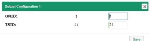
Edit ONID (Original Network Identifier) and TSID (Transport Stream Identifier) fields with the desired values for that carrier and push Save button.
