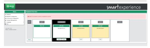
This screen shows the whole headend schematically. The essential information of each module inserted in the base-plate is displayed. The master module always corresponds with the module inserted in slot 2, and it appears in white on black background. The remaining modules appear on white background.
