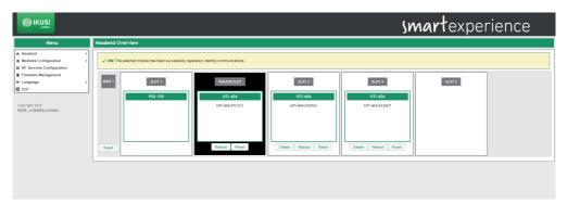
If, for any reason, you want to unregister a module of the headend, you must push the Delete button. The module will be displayed in yellow background, indicating that has been unregistered correctly.
