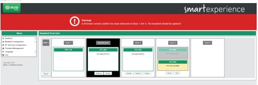
A module with two possible configurations is displayed: one in grey background, corresponding to the previous module that was already registered in the headend, and another one in yellow background, corresponding to the configuration of the new module pending registration.
