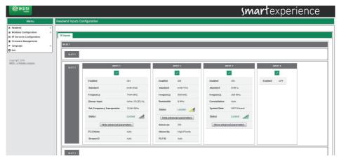
Tuning status (Locked or Unlocked) will appear in each of the inputs. Also, an icon indicating the level of signal and its quality, where red is bad quality, yellow medium quality and green good quality, will be displayed.
