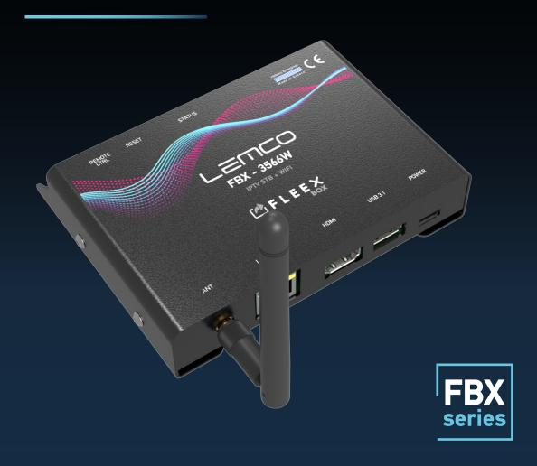
Boasting a high-performance quad-core A55 CPU clocked at 2GHz, coupled with 2GB DDR4 memory and a Mali-G52 GPU, this device is a powerhouse of efficiency and speed. Its specialized lightweight Linux OS ensures peak performance and ultra-fast booting.
