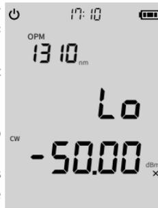
The units of Absolute Power, Relative Power and Linear Power are dBm, dB, mW/nW. The conversion relationship is as follows:  $P_{Abs.power} = 10 \lg P_{Lin.power} / 1mW$        $P_{Rel.power} = P_{Abs.power} - P_{Ref.power}$
