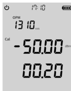
Note: The calibration and adjustment range of the power meter is from -6dBm to +6dBm.
