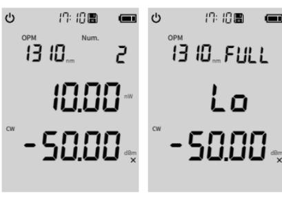
Note: When there are 1000 pieces of data saved, the interface will display "FULL" when saving again. It is recommended to export the data in time and delete the internal data of the instrument, otherwise it cannot continue to save.
