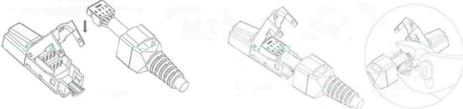
⑥ Close plug cover, make sure the drain wire is in proper contact with grounding clip on plug.
