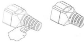
③ Fan out all four twisted pairs, following the color coding label and allocate each conductor into proper slots on wiring cap. Trim the ends of conductors.
