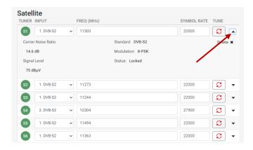
Carrier Noise Ratio: Shows the carrier to noise ratio of the input signal
