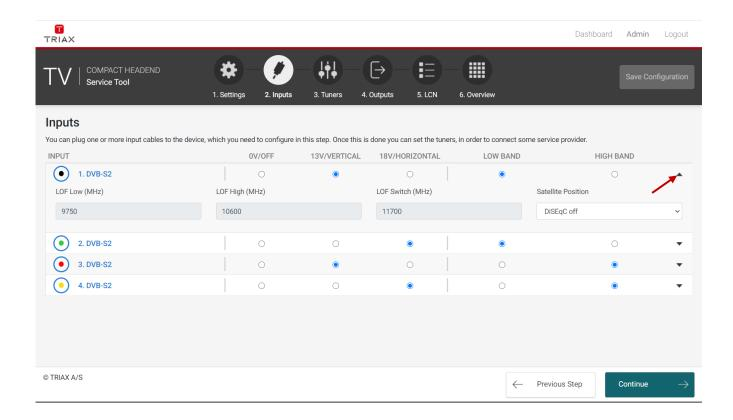
When you press the expand button you can open the DiSEqC settings:
