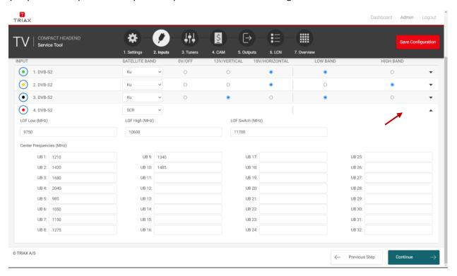
The TDcH SCR functionality supports up to 32 User bands per SCR input. The center frequencies can be entered on the table as shown in the screen shoot.
