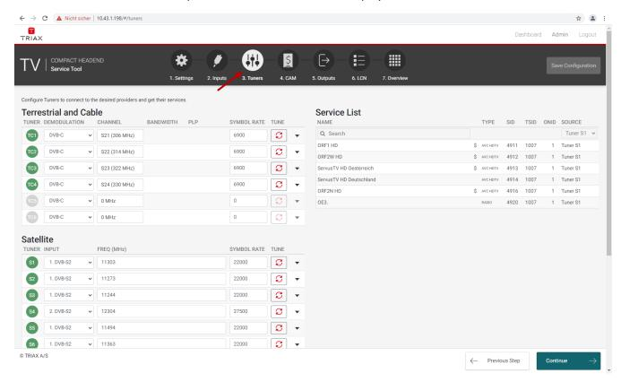
The "Tuner" folder shows all input tuners. The colour of the tuner number shows the status of each tuner.
