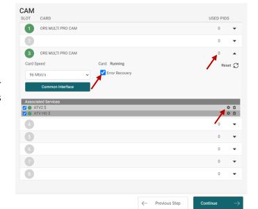
The Error Recovery function does a constant monitoring of the signal transmission status through the CA module. The CA module is automatically reset if the signal transmission fails. When a CA module is reset, the signal transmission is interrupted for all the services associated with that CA module. The "Error Recovery" checkbox should not be enabled for services where signals are not transmitted on a 24-hour basis.
