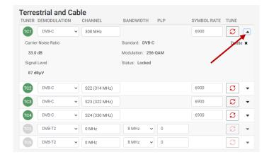
Carrier Noise Ratio: Shows the carrier to noise ratio of the input signal
