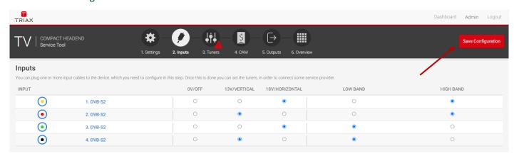
An important button when you change your configuration of the headend system is the "Save Configuration" button placed in the upper right-hand corner of the TDX Service Tool window.
