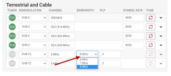
4. If the tuner is used as DVB-C than please select the required symbol rate:
