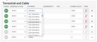
3. If the tuner is used as DVB-T/T2 than please select the required cannel bandwidth and PLP number:
