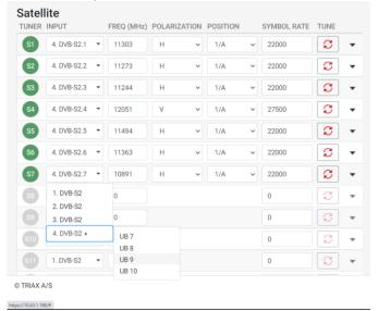
You have to select the SCR user band and the Polarisation and Satellite position.
