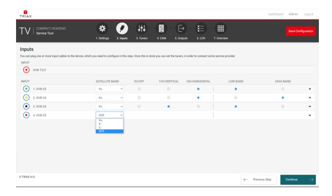
When you press the expand button you can open the SCR and LOF settings:
