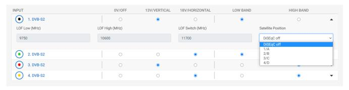
DiSEqC supports four satellite positions. Please select the desired position if required.
