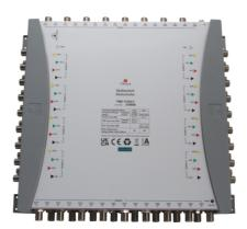
Cascade multiswitch for 4 Satellite positions with 17 inputs and 17 trunk outputs, suitable for distributing satellite and terrestrial signals in small to large sized systems. Available with 32 subscriber outputs and powered by the TMS PSU external power supply either directly or via the SAT trunk lines.
